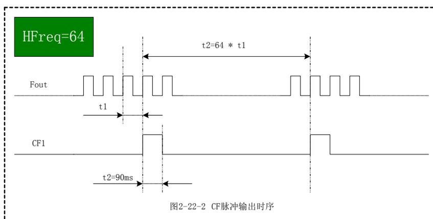
图2-22-2 CF脉冲输出时序
